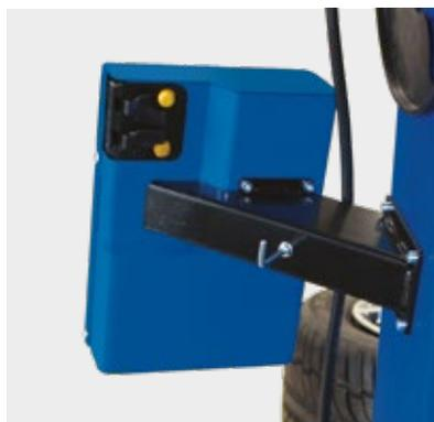
The buttons on the back allow not to move the look of the operator from the tyre.
